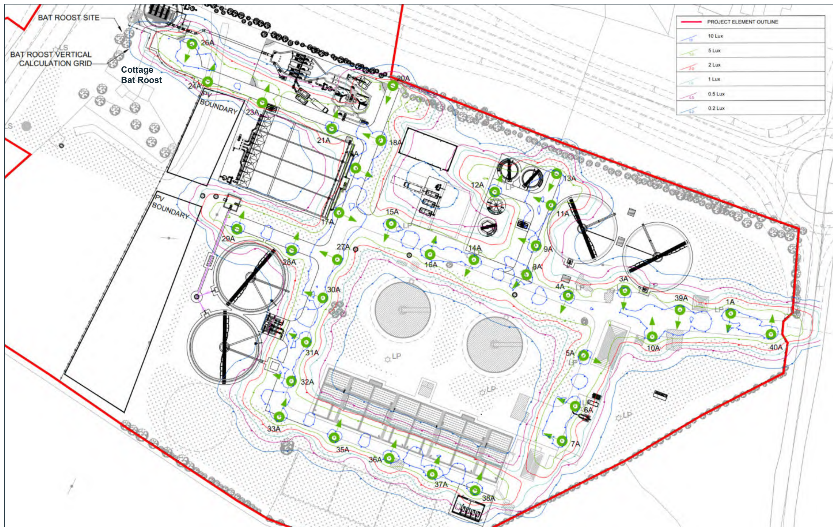
Figure 5-19 - Operational lighting plan, see full scale drawing 5161805_EWE_DR_MOR_1300 included in the planning pack.
