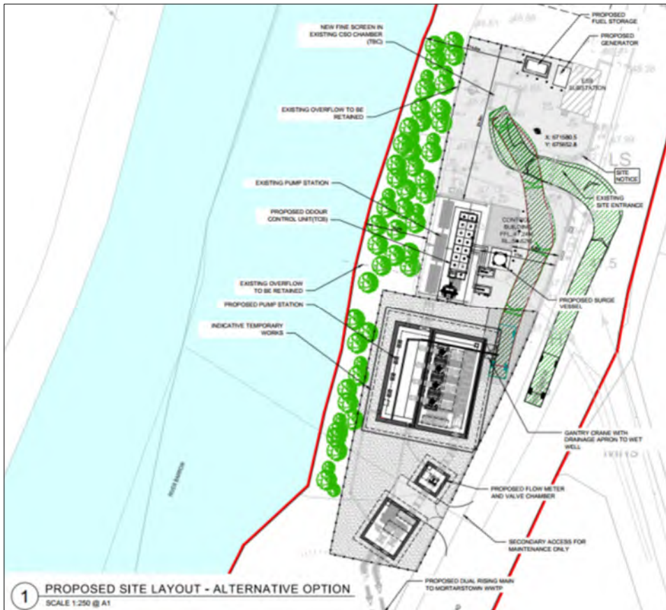
Figure 3-4 - Rectangular Pump Station - Site Layout Option
